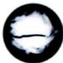
Internal Crack in a Copper Coin is Revealed by X-Radiography
